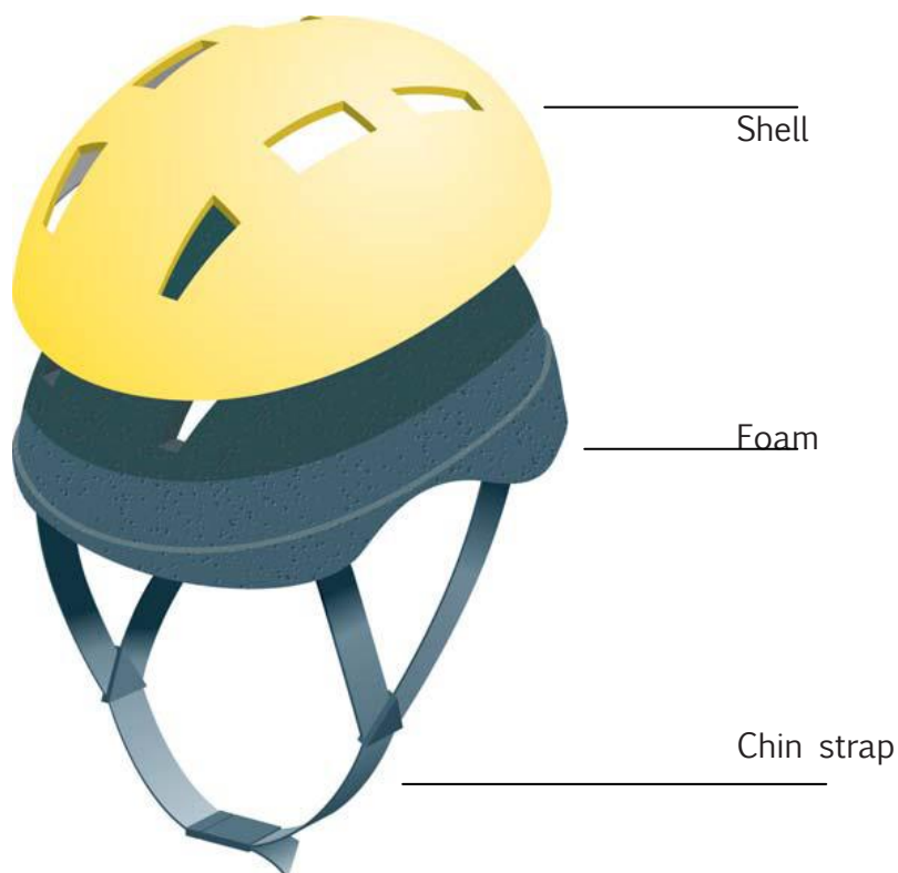
Figure 9.3 Expanded polymer foam helmet
